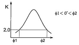
Contrast ratio K vs viewing angle  $\phi$
