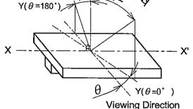
Note 2: Definition of viewing angle  $\phi 1$  and  $\phi 2$
