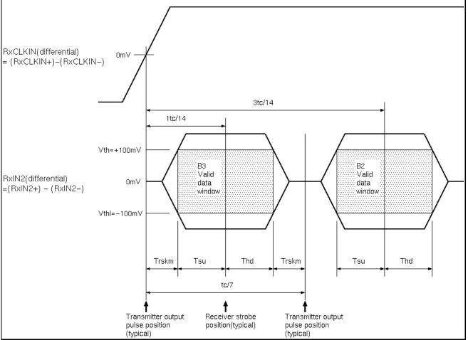
**Note :** Tsu and Thd are internal data sampling window of receiver. Trskm is the system skew margin; i.e., the sum of cable skew, source clock jitter, and other inter-symbol interference, shall be less than Trskm.
