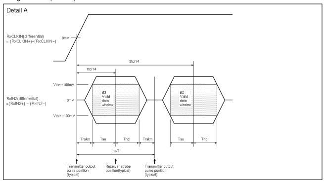
**Note:** Tsu and Thd are internal data sampling window of receiver. Trskm is the system skew margin; i.e., the sum of cable skew, source clock jitter, and other inter-symbol interference, shall be less than Trskm.
