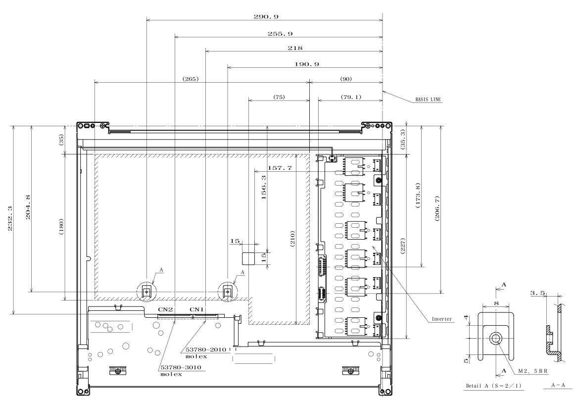
Note1: The torque for mounting screws should never exceed 0.45N·m.
