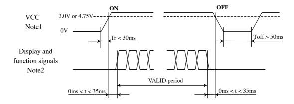
Note1: In terms of voltage variation (voltage drop) while VCC rising edge is below 3.0V in "VCC = 3.3V" or 4.75V in "VCC = 5.0V", a protection circuit may work, and then this product may not work.
