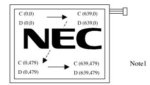
Figure 1. Normal scan (DPS: Low or Open)
