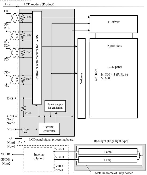
Note1: Connections between GND (Signal ground), FG (Frame ground) and VBLC (Lamp low voltage terminal) in the LCD module
