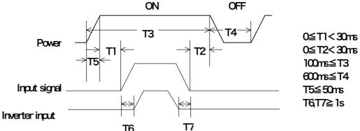
T6 T7 note ··· The time regulations from T1 to T7 are defined as a changing point 10% of the amplitude of "Input signal" and "Power", and 90%
