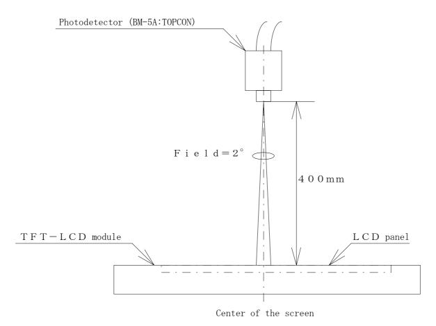
Fig. 3 Optical characteristics measurement method
